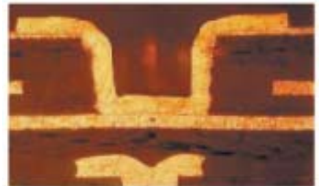
0.009" x 0.009" blind via (230 x 230 \mu\text{m} )
